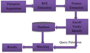
Fig. 3.General block diagram of palmprint recognition system
