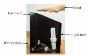
Fig. 8. Touchless device used to capture hand images [touchless6]
